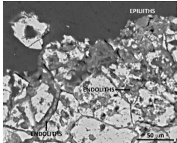
**Fig. 2:** Back-scattered electron scanning microscope image of fungi colonizing the surface (epiliths) and interior (endoliths) of dolostones.
