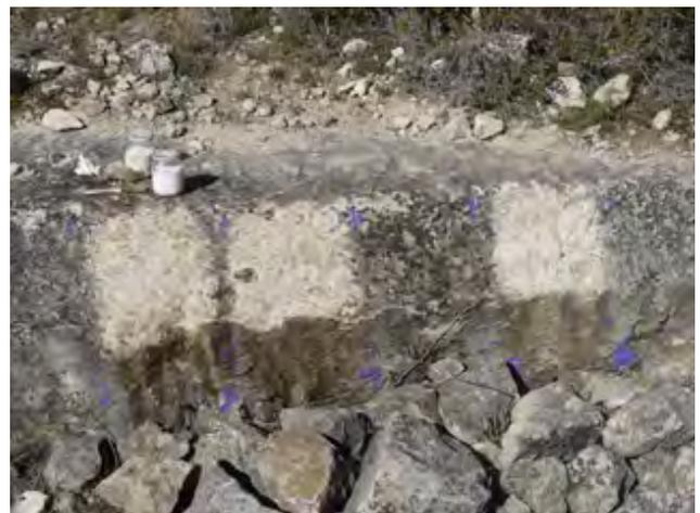
**Fig. 1: Set of experiments designed to test new cleaning treatments at Redueña Quarry (Madrid, Spain).**
