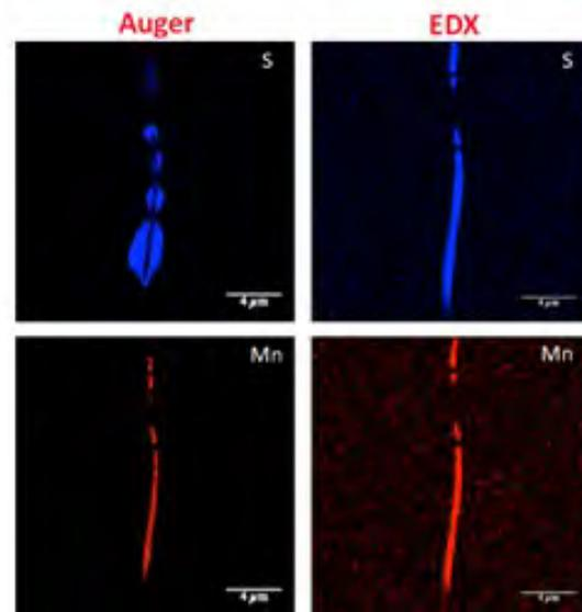
**Figure 1:** Mn and S elemental maps of polished 1018 carbon steel obtained using an Auger electron detector and, for comparison, an X-ray detector.
