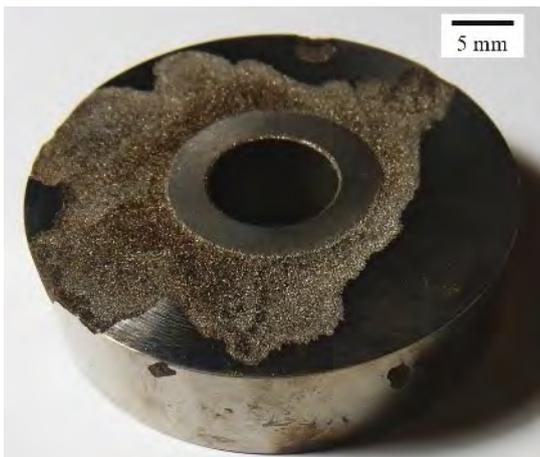
Localised corrosion of Monel immersed in sea water, evidence suggests that the rapid corrosion (~3 mm/yr) was due to MIC
