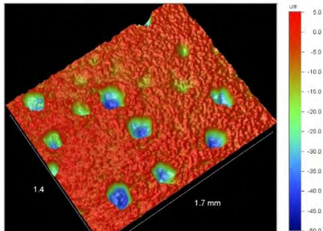
3D optical profile image showing the localised corrosion of carbon steel from laboratory study using sulfate reducing
